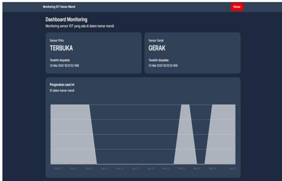
Figure 3. Display of Door Open and Motion Detected Operational Conditions
