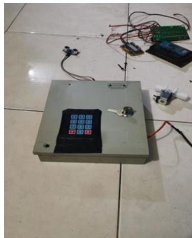
Figure 7. 4x4 Keypad Sensor Testing
